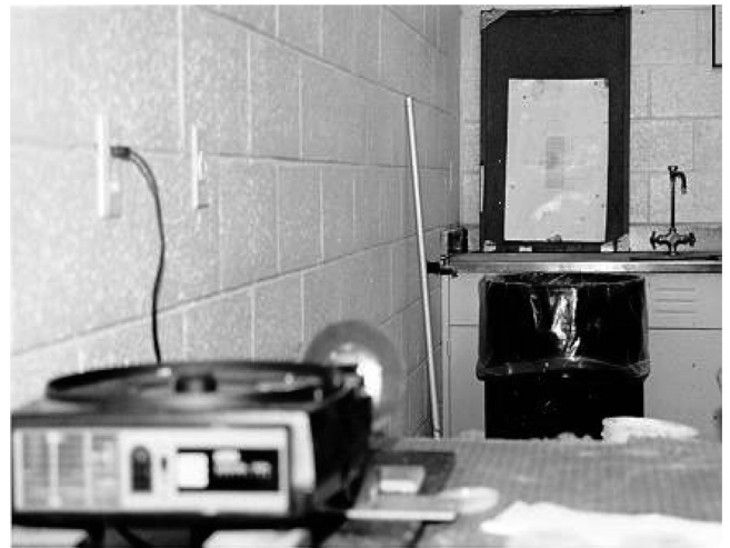
Fig. 2.2—Test setup for ASTM C 827 with slide projector and lens (disk in front of projector) in foreground and calibrated chart on wall background.
